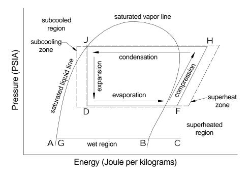
The P-E chart is an important tool in understanding the property changes that take place during each phase of the cycle and provides a graphical means of study. Horizontal lines on the P-E chart are lines of constant pressure and vertical lines are lines of constant enthalpy or heat energy.
